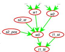
• W0 depends only on whether there is power in w1, whether there is power in w2, the position of switch s2  $(S2\_pos)$ , and the status of switch s2  $(S2\_st)$ .
